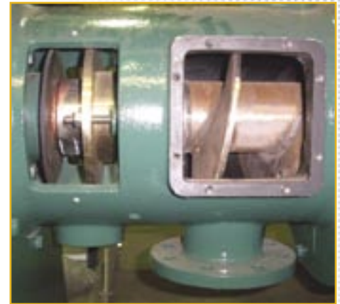
Feed zone inspection and access hatch
